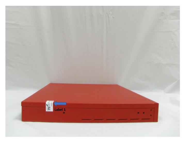
Figure 16: M500 Tamper Evident Label 1 Placement
