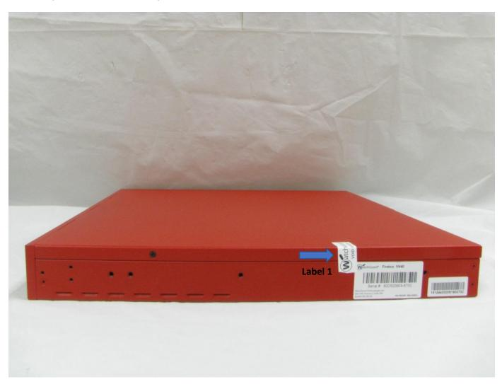
Figure 17: M440 Tamper Evident Label 1 Placement
