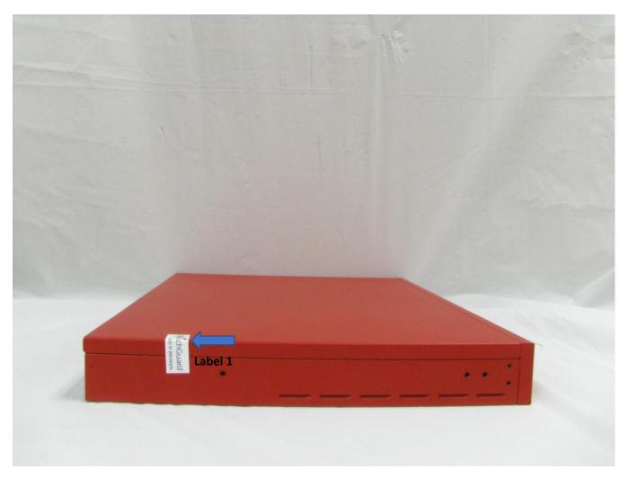
Figure 15: M400 Tamper Evident Label 1 Placement
