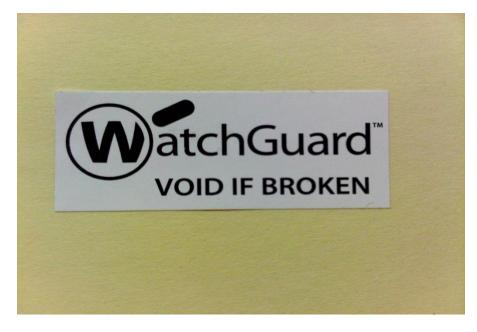
Figure 12: WatchGuard Firebox Tamper Evident Label
