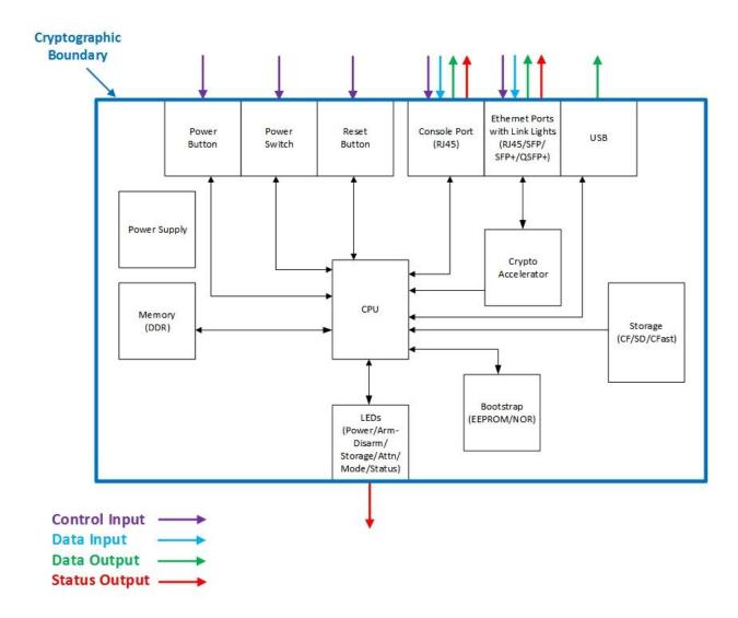
Figure 1: Cryptographic Module Block Diagram
