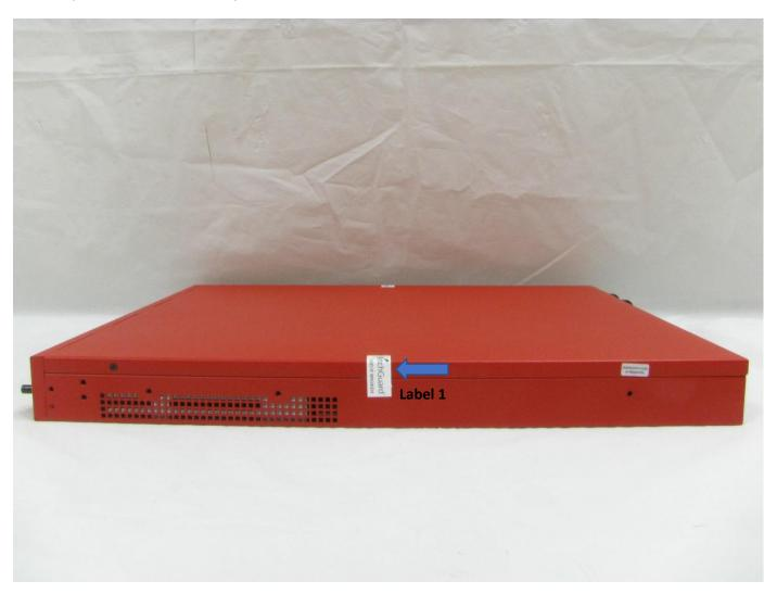
Figure 20: M4600 Tamper Evident Label 1 Placement
