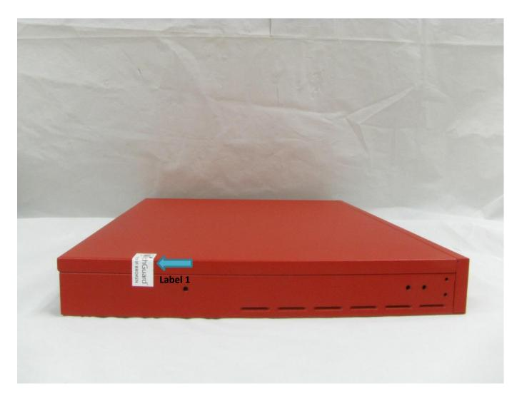
Figure 14: M300 Tamper Evident Label 1 Placement
