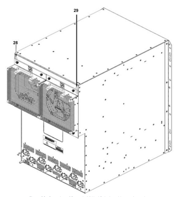
Figure 23 - Rear view of Brocade MLXe-16 device with security seals
