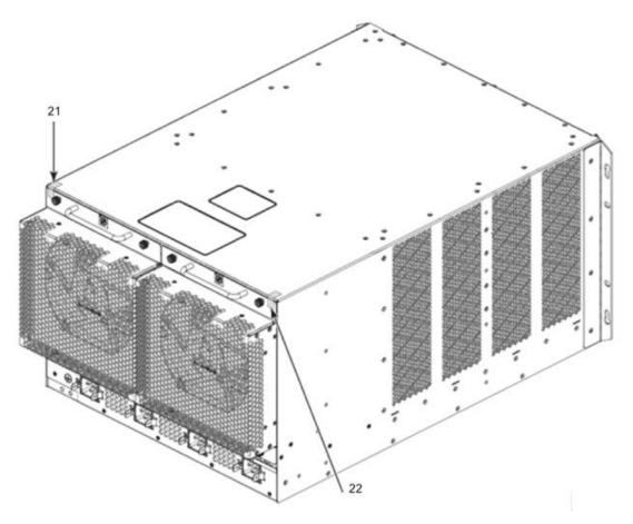
Figure 21 - Rear view of Brocade MLXe-8 device with security seals
