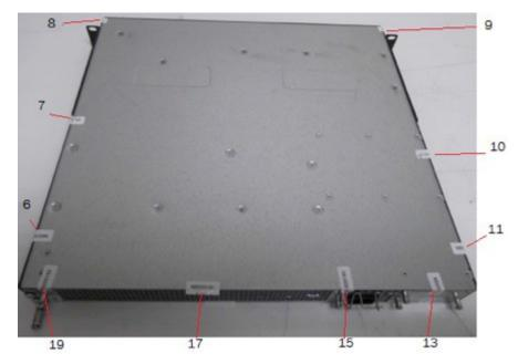
Figure 51 - Bottom view of Brocade CES 2024C-4X device with security seals
