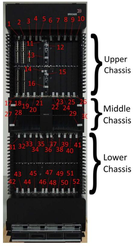
Figure 28 - Front overview of MLXe-32 Configuration 2 with tamper labels
