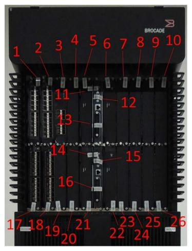
Figure 29 - Front overview of MLXe-32 Configuration 2 with tamper labels
