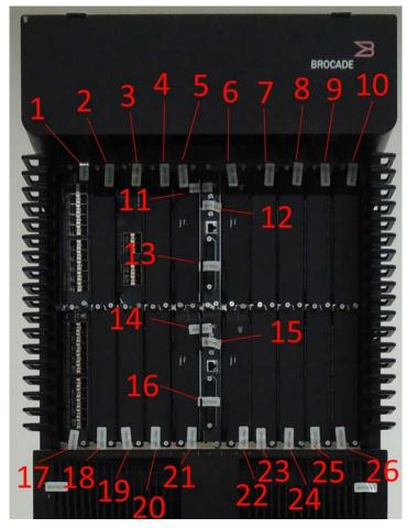
Figure 25 - Front upper chassis of MLXe-32 Configuration 1 with tamper labels
