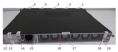
Figure 55 - Rear side view of Brocade CES 2024F-4X device with security seals
