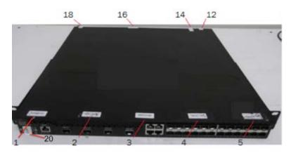
Figure 52 - Top front view of Brocade CES 2024F-4X device with security seals
