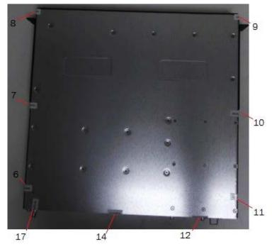
Figure 41 - Bottom view of Brocade CER 2024C-4X-RT device with security seals
