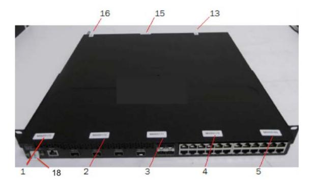
Figure 37 - Top front view of Brocade CER 2024C-4X-RT device with security seals
