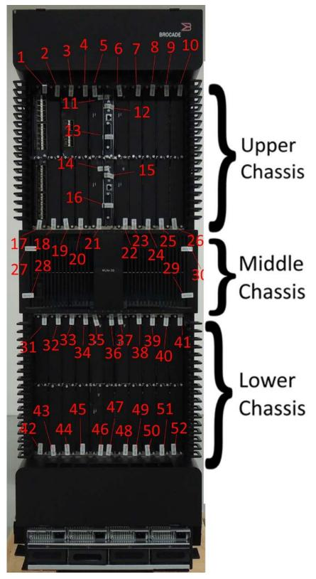
Figure 24 - Front overview of MLXe-32 Configuration 1 with tamper labels
