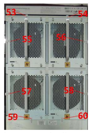
Figure 35 - Back upper chassis of MLXe-32 with tamper labels
