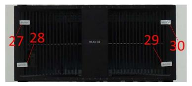
Figure 30 - Front middle chassis (grill) of MLXe-32 Configuration 2 with tamper labels
