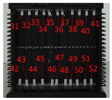
Figure 27 - Front lower chassis of MLXe-32 Configuration 1 with tamper labels
