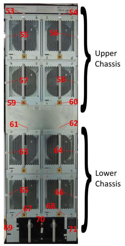
Figure 34 - Back overview of MLXe-32 with tamper labels
