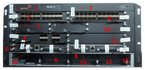
Figure 18 - Front view of Brocade MLXe-4 with security seals
