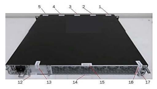
Figure 40 - Rear view of Brocade CER 2024C-4X-RT device with security seals
