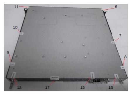
Figure 46 - Bottom view of Brocade CER 2024F-4X-RT device with security seals
