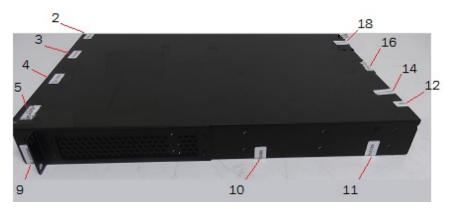
Figure 48 - Right side view of Brocade CES 2024C-4X device with security seals
