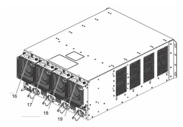
Figure 19 - Rear view of Brocade MLXe-4 device with security seals
