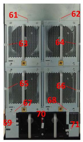
Figure 36 - Back lower chassis of MLXe-32 with tamper labels
