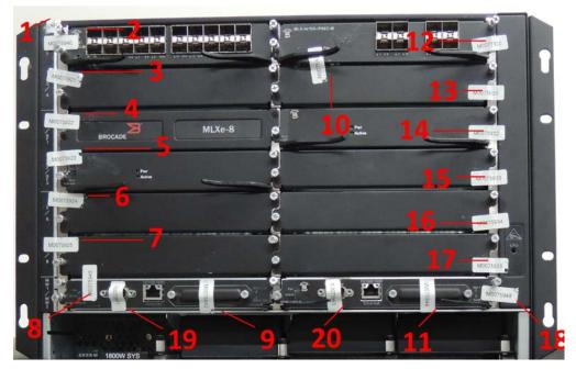
Figure 20 - Front view of Brocade MLXe-8 device with security seals
