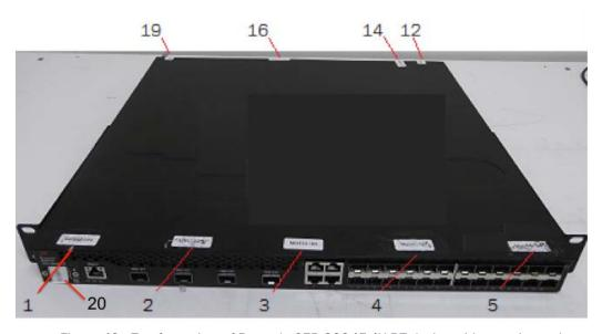
Figure 42 - Top front view of Brocade CER 2024F-4X-RT device with security seals
