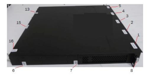
Figure 39 - Left side view of Brocade CER 2024C-4X-RT device with security seals
