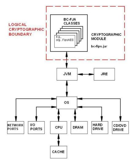
Figure 2 – Module's Logical Cryptographic Boundary
