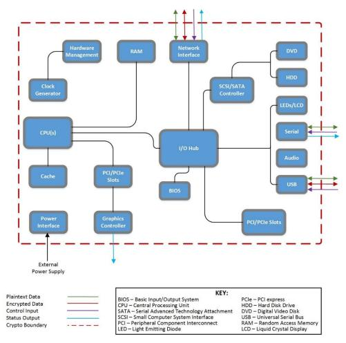
Figure 1 – Hardware Block Diagram
