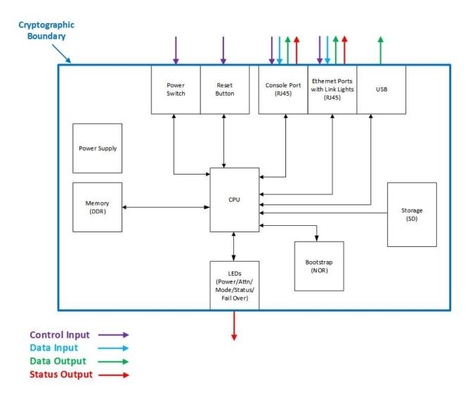
Figure 1: Cryptographic Module Block Diagram
