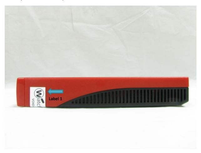
Figure 18: T30-W Tamper Evident Label 1 Placement
