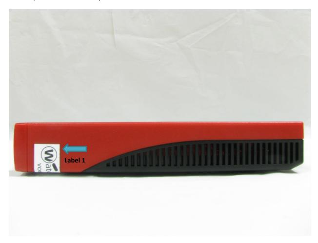
Figure 17: T30 Tamper Evident Label 1 Placement
