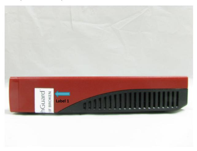
Figure 15: T10 Tamper Evident Label 1 Placement
