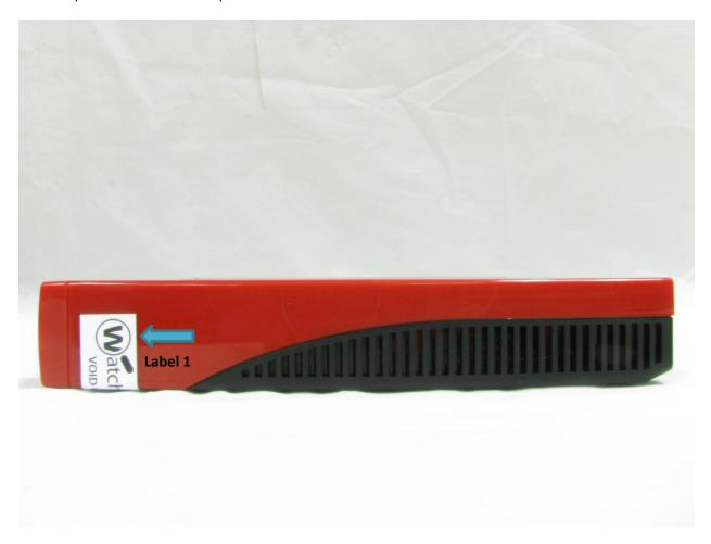
Figure 20: T50-W Tamper Evident Label 1 Placement
