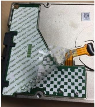
Figure 2: Tamper Evident Security Label on PCBA Showing Evidence of Tampering
