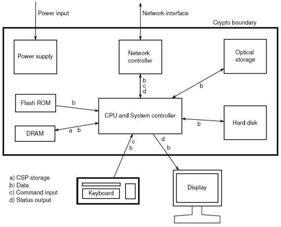
Figure 2 - Cryptographic Module Physical Boundary
