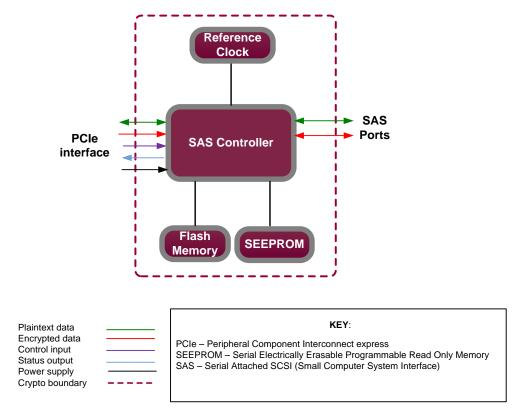
Figure 1 – Unity 12 Gb/s SAS I/O Module with Encryption Block Diagram
