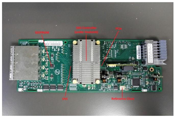
Figure 2 – Top view of Pluggable I/O SAS Module
