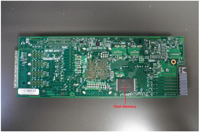
Figure 3 – Bottom view of Pluggable I/O SAS Module
