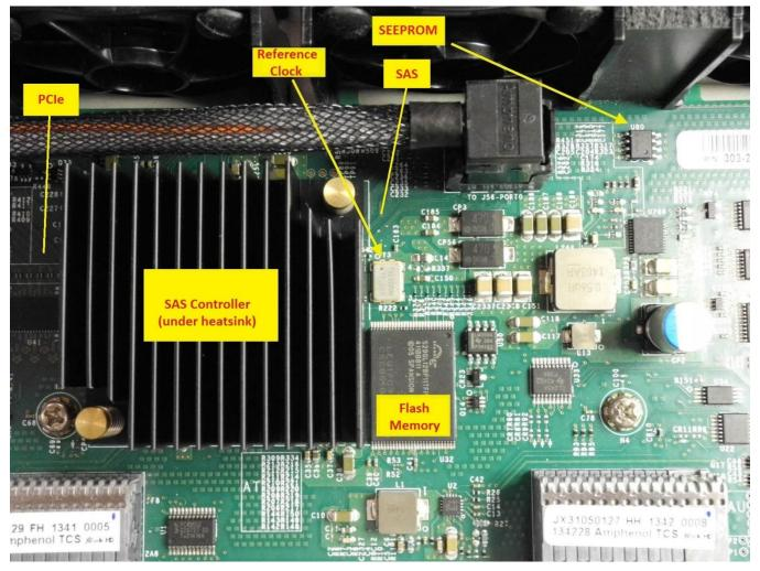
Figure 4 – Top view of Storage Processor SAS Module
