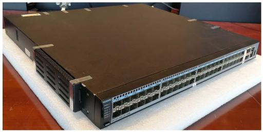
Figure 2-3 S6720-54C-EI-48S-AC (Top, Left, Front)
