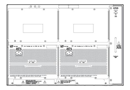
FIGURE 5 - BACK OF A 5412R ZL2 SWITCH WITH TWO POWER SUPPLIES
