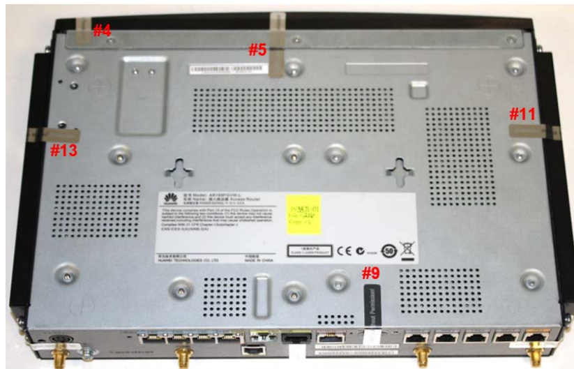
Figure 26: Bottom and Front Plate Seals
