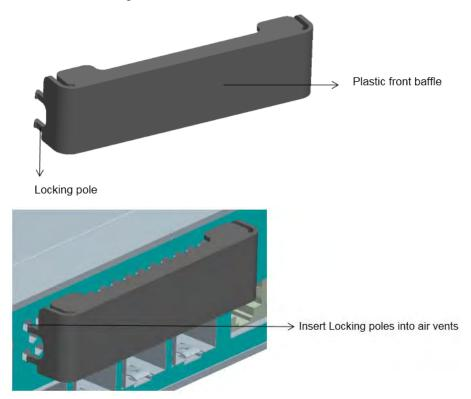
Figure 7-8: Install Baffle into Front Panel
