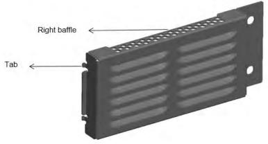
Figure 7-5: Insert the two tabs on the baffle into air vents on the right side of the switch.
