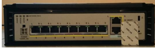
Figure 16 ASA 5506-X and ASA 5506W-X Rear TEL Placement
