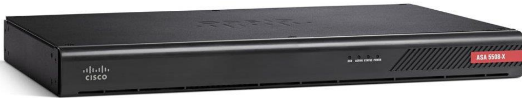
Figure 6 ASA 5508-X and ASA 5516-X Appliances Front Panel
