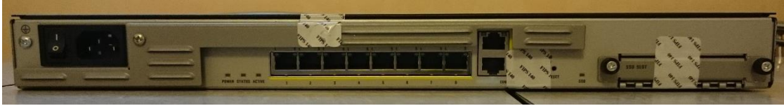
Figure 44 ASA 5516-X Rear TEL Placement
