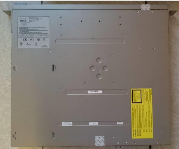
Figure 42 ASA 5515-X Bottom TEL Placement
