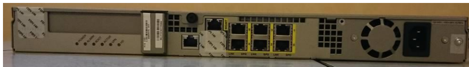
Figure 39 ASA 5515-X Rear TEL Placement
