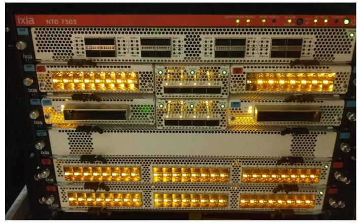
Figure 1 – NTO 7303 Chassis P/N 991-0082-01 (Front view; fully populated)
