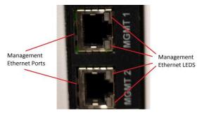
Figure 16 – Management Ethernet Ports and LEDs
