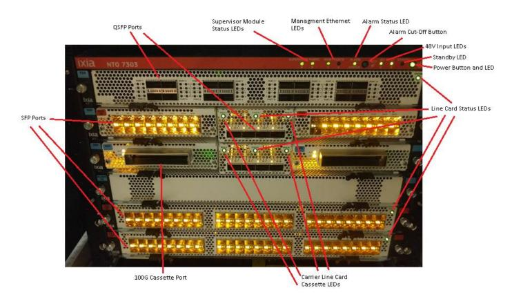
Figure 14 – NTO 7303 Front Ports and Interfaces
