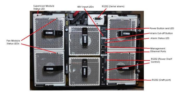
Figure 15 – NTO 7303 Rear Ports and Interfaces
