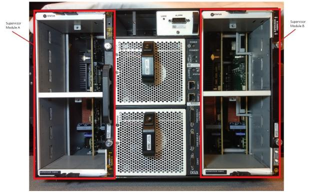
Figure 3 – NTO Supervisor Module P/N 992-0059-01 (with fan modules removed)
