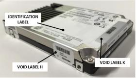
OUTER SHEET is an opaque seal covering some holes of the top cover. It cannot leave "VOID" message, but leaves the evidence of the cut.
