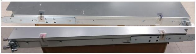
Figure 2 - Tamper Evidence Label Locations
