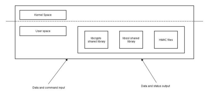
Figure 2: Software Block Diagram (the cryptographic boundary includes the HMAC integrity files)
