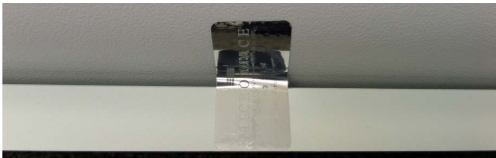
Figure 4 – Tamper-Evident Seal Applied over Small Gap Between Metal Backing and Plastic Cover
