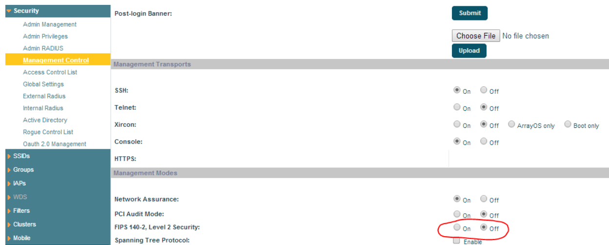
Figure 10 – Security Management Control Window
