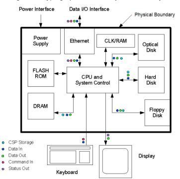
Figure 2: Cryptographic Module Physical Boundary
