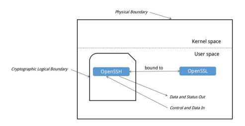
The module is aimed to run on a general purpose computer; the physical boundary is the surface of the case of the target platform, as shown in the diagram below:
