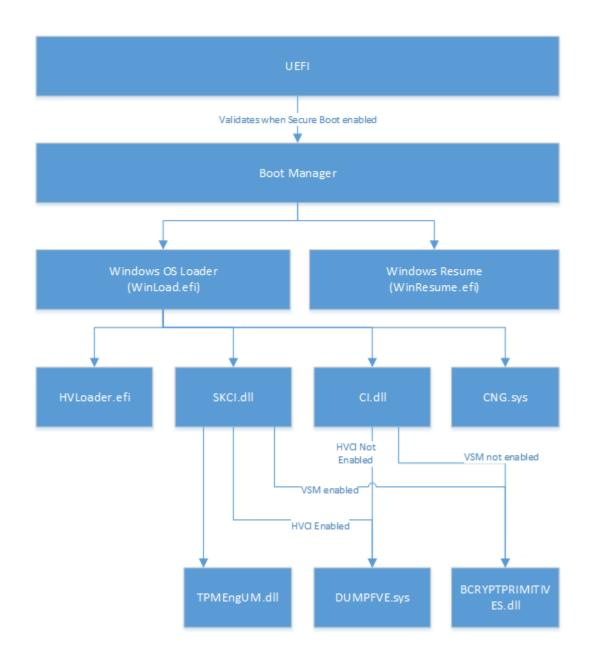
The integrity of the Code Integrity module is checked by the Windows Loader. The Code Integrity module is then, in certain configurations, responsible for checking integrity of every other user and kernel mode system binary as they are loaded.
