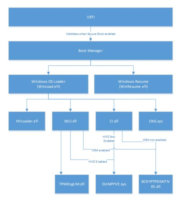
The integrity of Cryptographic Primitives Library is checked by Code Integrity or Secure Kernel Code Integrity before it is loaded into process memory.
