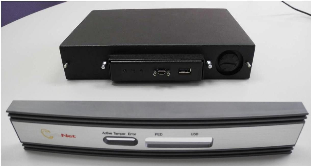
Figure 2-2. SafeNet Backup HSM (with front bezel removed) ..... 9
