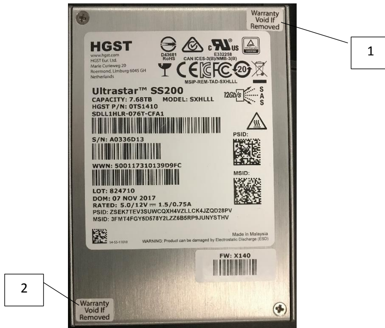
Figure 7. - Tamper-Evident Seal Locations on Top, SDLL1CLR-020T-CF, SDLL1DLR-960G-CF, SDLL1DLR-480G-CF, SDLL1DLR-800G-CF, SDLL1DLR-400G-CF, Version 1
