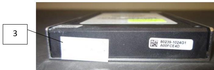
Figure 9 - Tamper-Evident Seal Location on Back Covering HDMI Port, SDLL1CLR-020T-CF, SDLL1DLR-960G-CF, SDLL1DLR-480G-CF, SDLL1DLR-800G-CF, SDLL1DLR-400G-CF, Version 1
