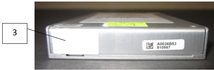
Figure 9 - Tamper-Evident Seal Location on Back Covering HDMI Port, SDLL1CLR-020T-CF, SDLL1DLR-960G-CF, SDLL1DLR-480G-CF, SDLL1DLR-800G-CF, SDLL1DLR-400G-CF, Version 1
