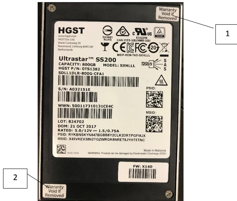
Figure 7. - Tamper-Evident Seal Locations on Top, SDLL1CLR-020T-CF, SDLL1DLR-960G-CF, SDLL1DLR-480G-CF, SDLL1DLR-800G-CF, SDLL1DLR-400G-CF, Version 1
