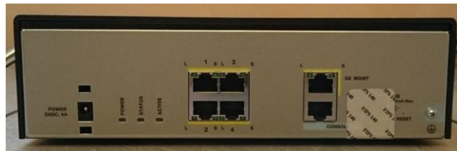
Figure 22 ASA 5506H-X Rear TEL Placement
