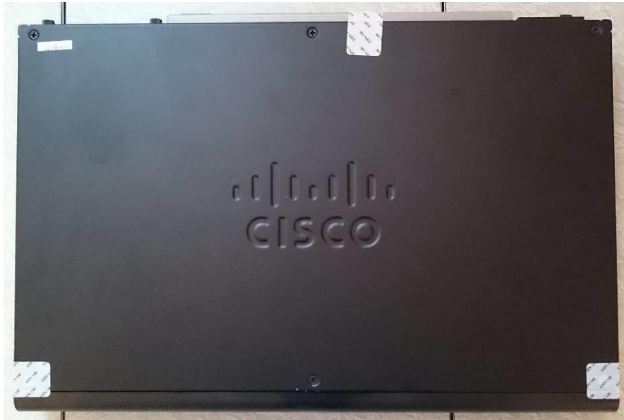
Figure 35 ASA 5516-X Top TEL Placement
