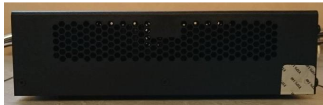
Figure 21 ASA 5506H-X Left Side TEL Placement
