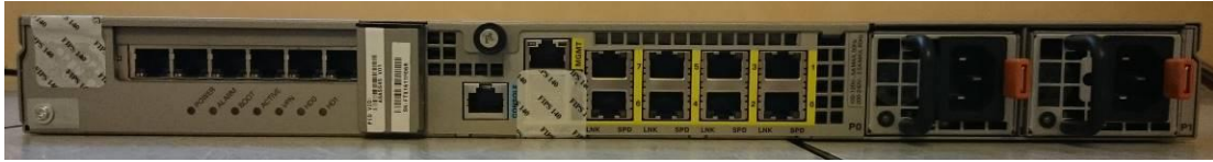
Figure 46 ASA 5545-X Rear TEL Placement
