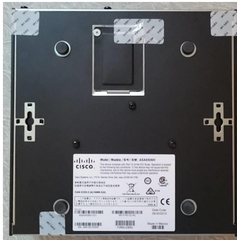
Figure 24 ASA 5506H-X Bottom TEL Placement
