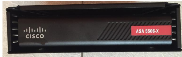
Figure 13 ASA 5506-X and ASA 5506W-X Front View
