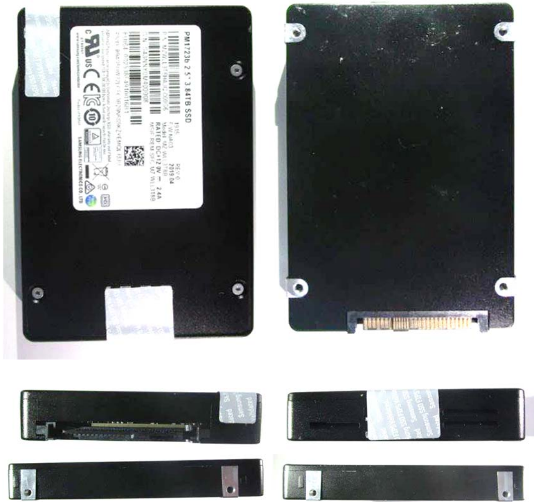
Exhibit 2 – Specification of the Samsung NVMe TCG Opal SSC SEDs PM1723b Series (MZWLL3T8HAJQ-000G6) Cryptographic Boundary (From top to bottom – Left to right: top side, bottom side, front side, back side, left side, and right side).
