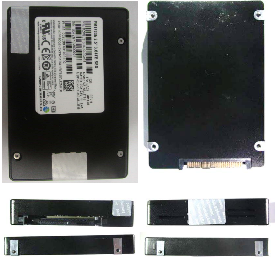
Exhibit 3 – Specification of the Samsung NVMe TCG Opal SSC SEDs PM1723b Series (MZWLL3T8HAJQ-00AG6) Cryptographic Boundary (From top to bottom – Left to right: top side, bottom side, front side, back side, left side, and right side).
