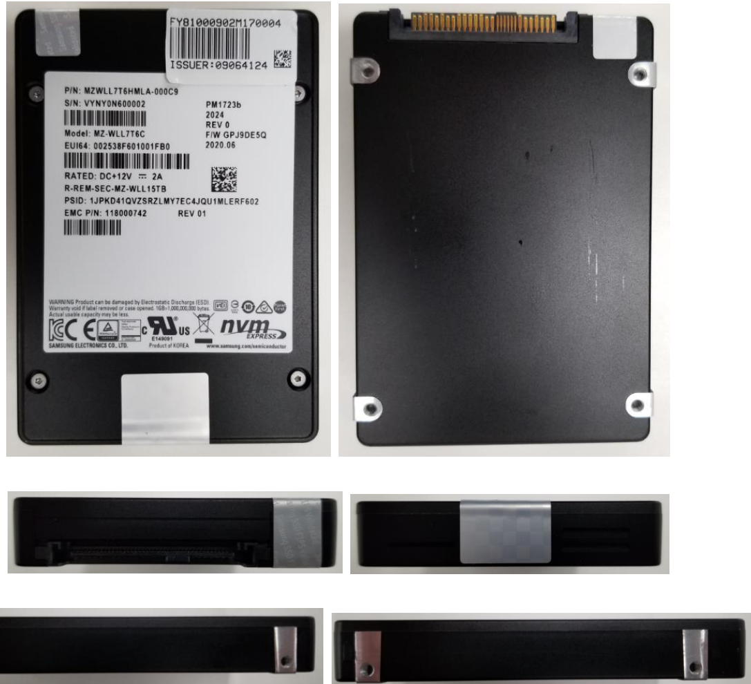
Exhibit 4 – Specification of the Samsung NVMe TCG Opal SSC SEDs PM1723b Series MZWLL7T6HMLA-000C9 Cryptographic Boundary (From top to bottom – Left to right: top side, bottom side, front side, back side, left side, and right side).
