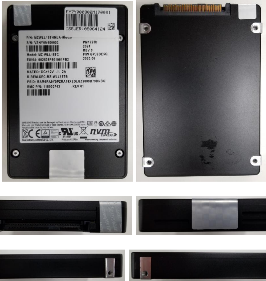
Exhibit 5 – Specification of the Samsung NVMe TCG Opal SSC SEDs PM1723b Series MZWLL15THMLA-000C9 Cryptographic Boundary (From top to bottom – Left to right: top side, bottom side, front side, back side, left side, and right side).
