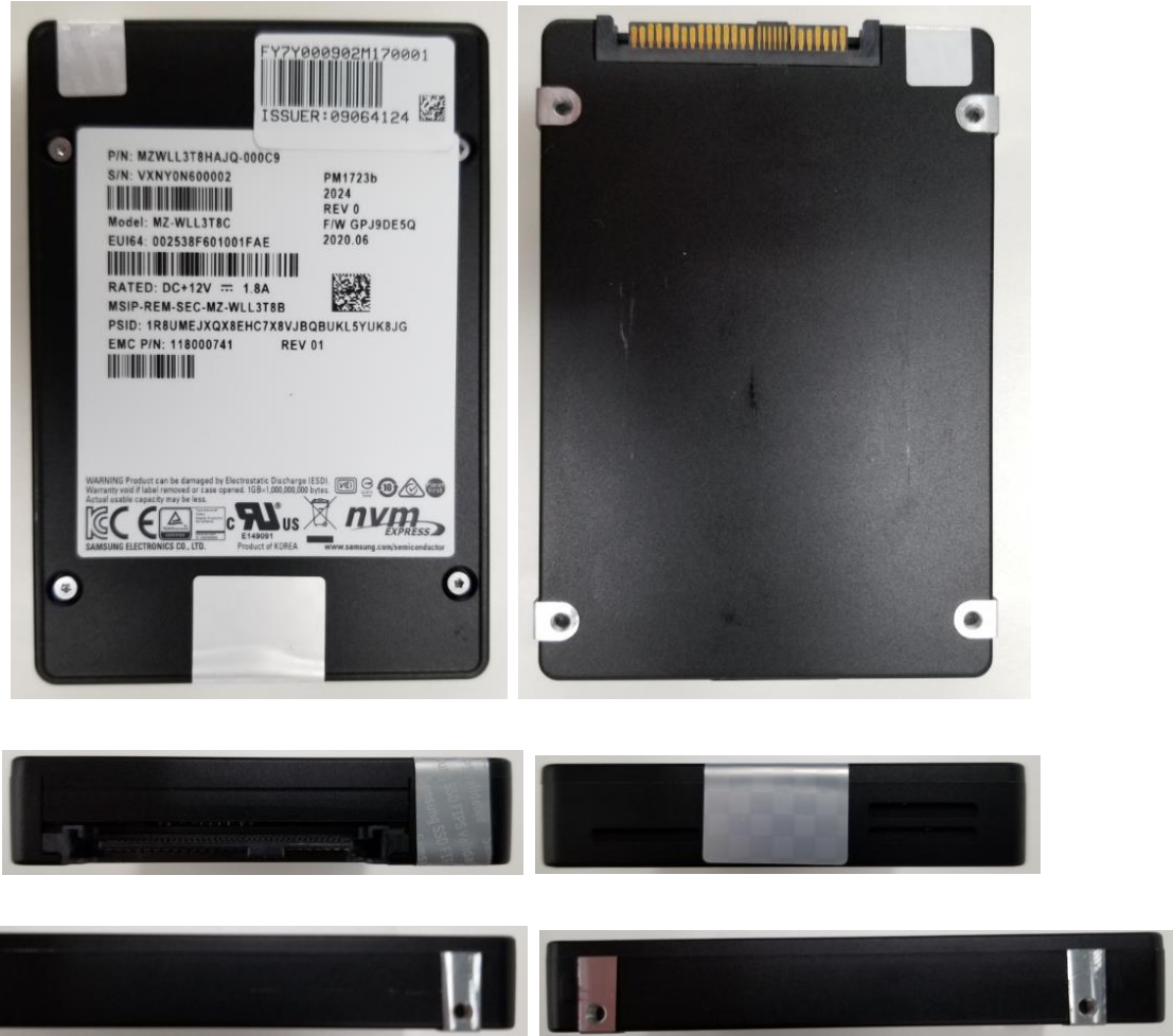
Exhibit 3 – Specification of the Samsung NVMe TCG Opal SSC SEDs PM1723b Series MZWLL3T8HAJQ-000C9 Cryptographic Boundary (From top to bottom – Left to right: top side, bottom side, front side, back side, left side, and right side).
