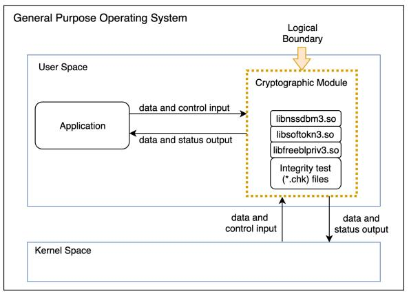
Figure 1: Logical cryptographic boundary.
