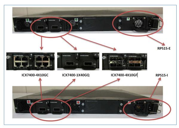
Figure 9 - Back side of the module ICX7450-48F with ICX7400-1X40GC, ICX7400-4X10GQ and ICX7400-4X10GF [DC power supply top; AC power supply bottom]
