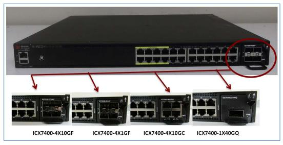
Figure 4 - Front/top side of the module ICX7450-24P with ICX7400-4X10GF, ICX7400-4X1GF, ICX7400-4X10GC and ICX7400-1X40GQ
