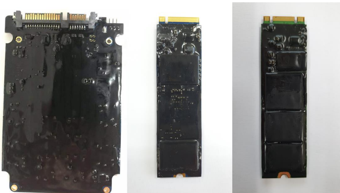
Figure 12 SATA 2.5" and M.2 Urethane/Epoxy Coating
