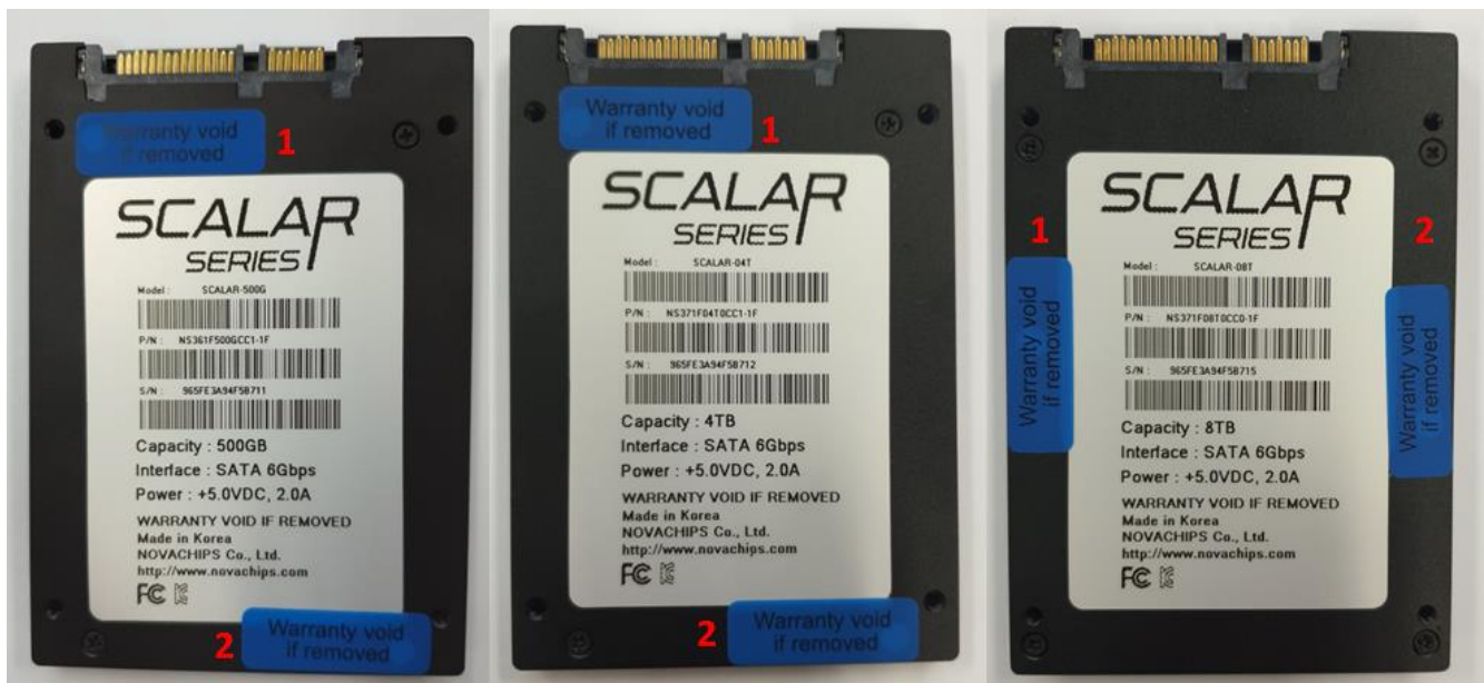
Figure 10 2.5" SATA enclosure and tamper evident label locations
