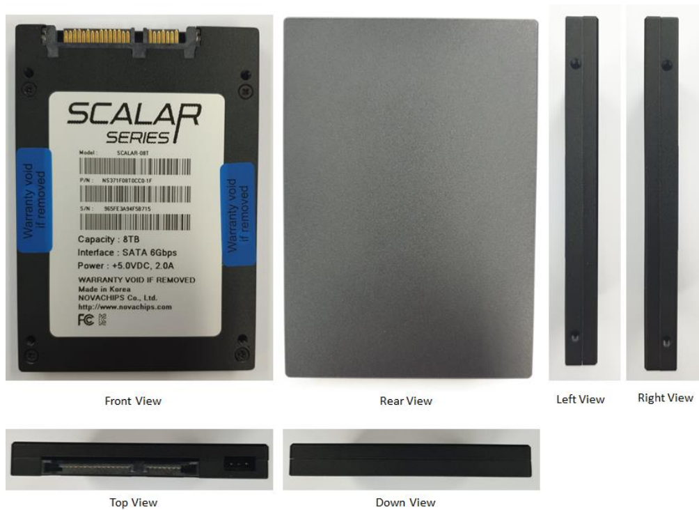
Figure 4 NS371F08TOCC0-1F 2.5" SATA 9.5mm SSD Module
