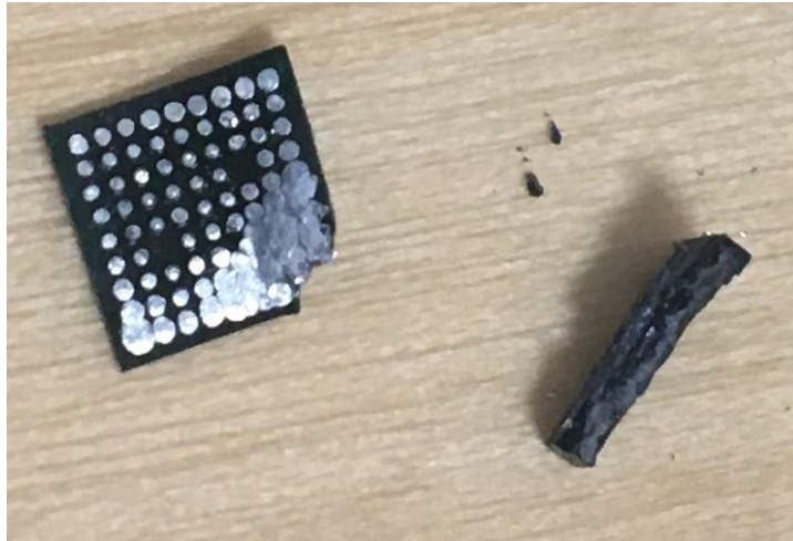
Figure 4- Tamper Evidence and damage to the module
