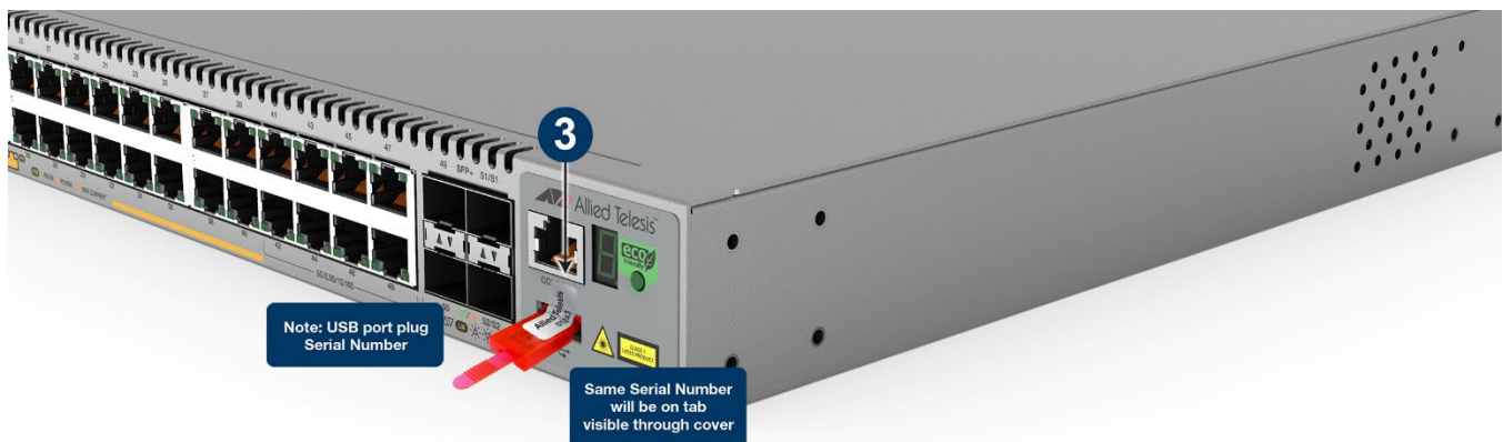
Figure 69: Location of USB Port Plug for x530-52GTXm
