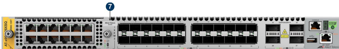
Figure 58: Tamper-Evident Seal Installed by Cryptographic Officer on XEM2
