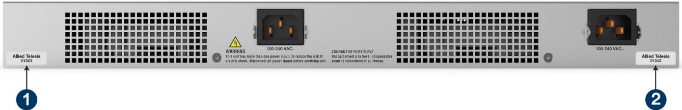
Figure 74: Tamper-Evident Seals on Rear of x530-28GPXm
