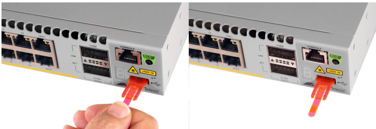
Figure 85: Putting USB Port Lock Tab into USB Port
