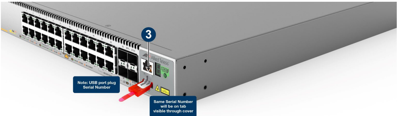
Figure 75: Location of USB Port Plug for x530-28GPXm
