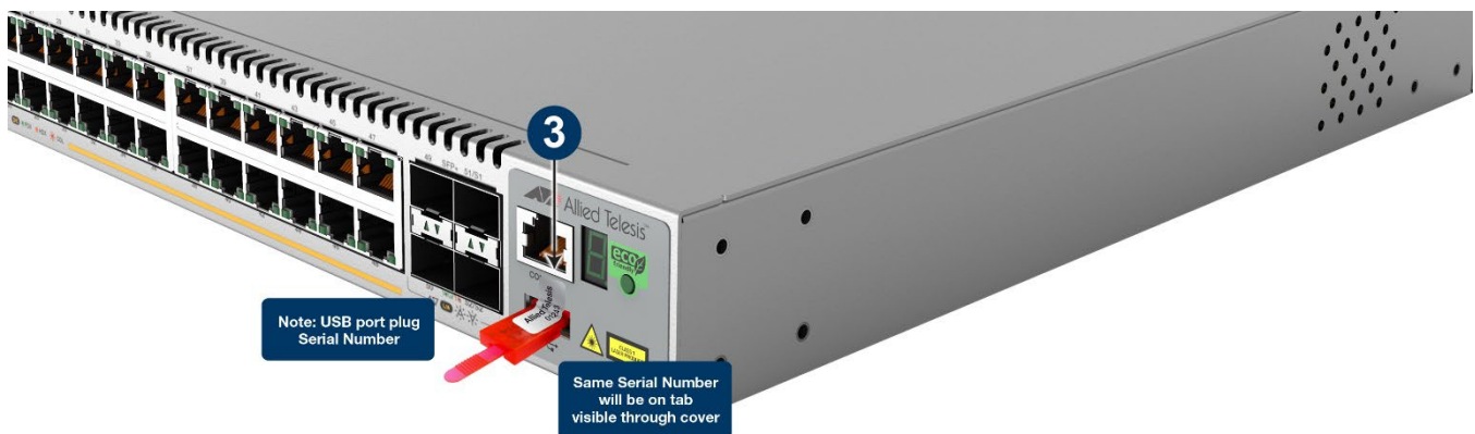
Figure 79: Location of USB Port Plug for x530L-52GPX
