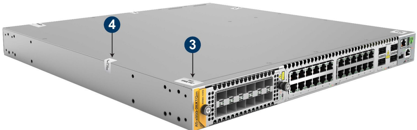
Figure 49: Tamper-Evident Seals on Top Left Side
