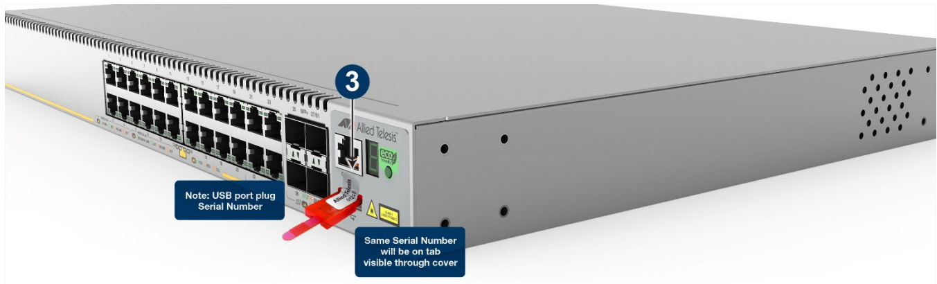
Figure 73: Location of USB Port Plug for x530-28GTXm
