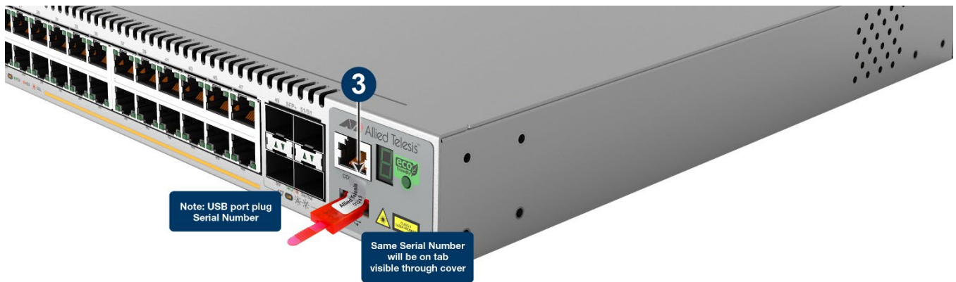
Figure 77: Location of USB Port Plug for x530L-52GTX
