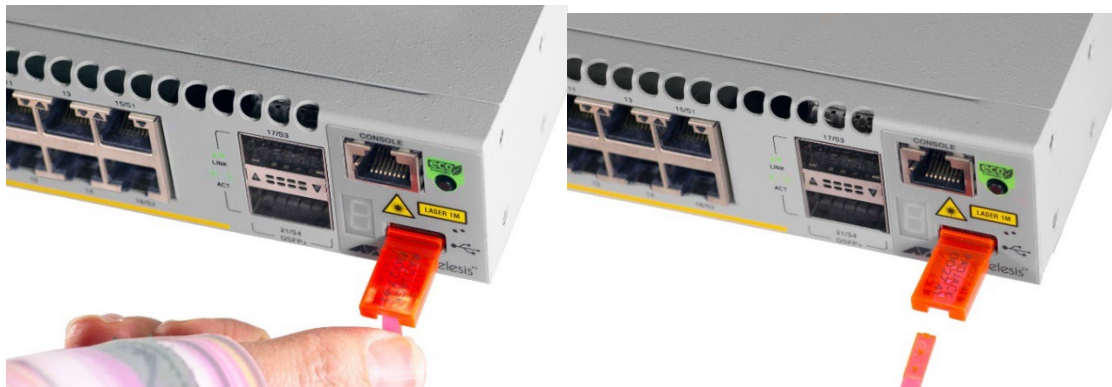
Figure 88: Breaking the Tab on USB Port Lock
