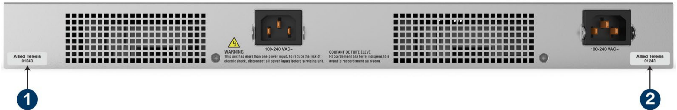
Figure 82: Tamper-Evident Seals on Rear of x530L-28GPX
