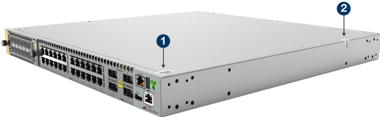
Figure 48: Tamper-Evident Seals on Top Right Side
