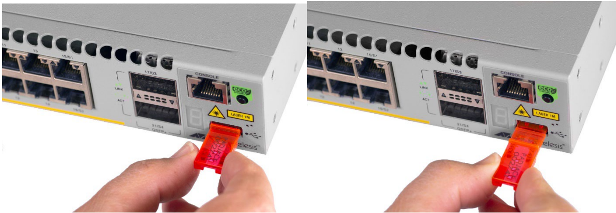
Figure 89: Removing the Housing from USB Port Lock
