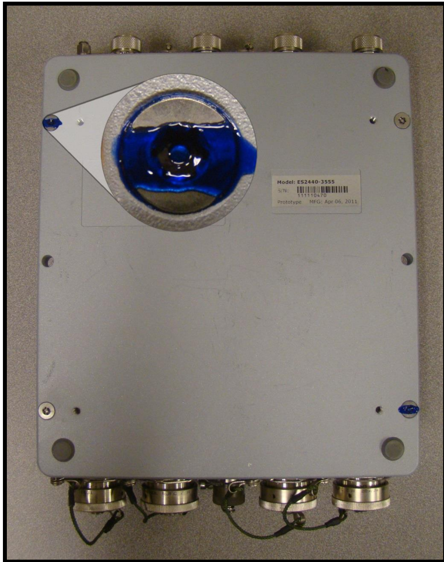
Figure 2: ES2440 Tamper Evidence (2 screws)
