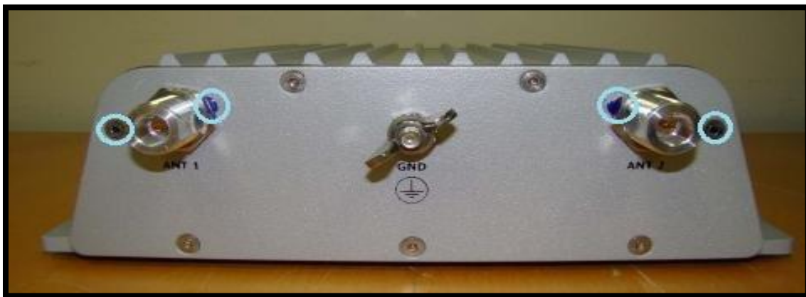
Figure 7 ES520 Version 2 (Rear) Tamper Evidence (4 screws)
