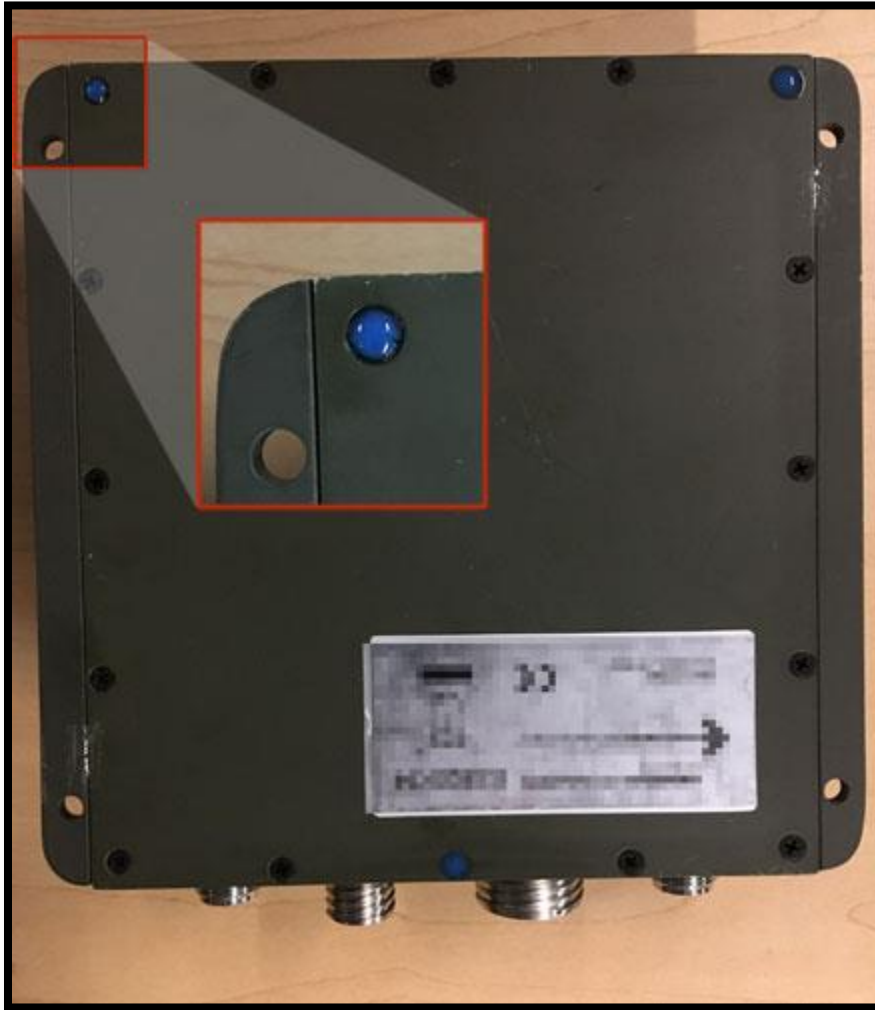
Figure 3: ES820 Tamper Evidence (3 screws)
