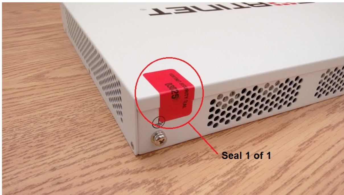
Figure 4 - FortiGate-201E external enclosure seal, top, rear
