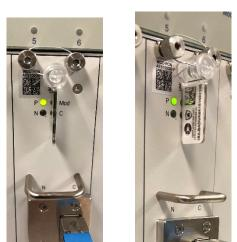
When the WCC-PCN-AES100GB-F card is installed in a 1U chassis, the two cross-drilled mounting screws that are supplied at the bottom front position of the card must be moved to secure the neighboring cards or blank panels. This
