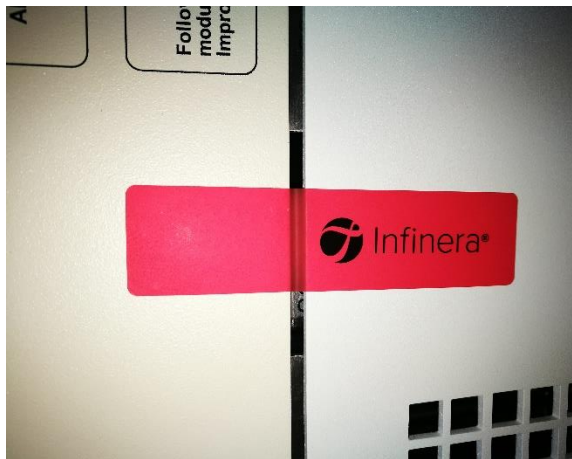
Figure 4 - Tamper-evident label: intact
