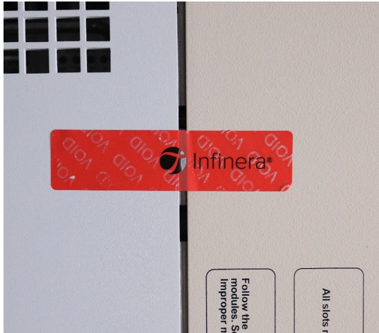
Figure 5 - Tamper-evident label: broken (normal view)
