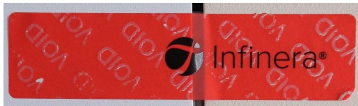
Figure 6 - Tamper-evident label: broken (close-up view)
