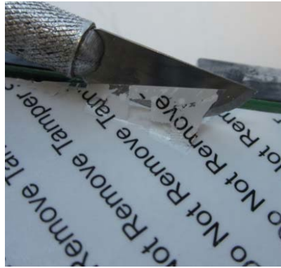
Figure 6: Tamper Evidence on Tamper Seal
