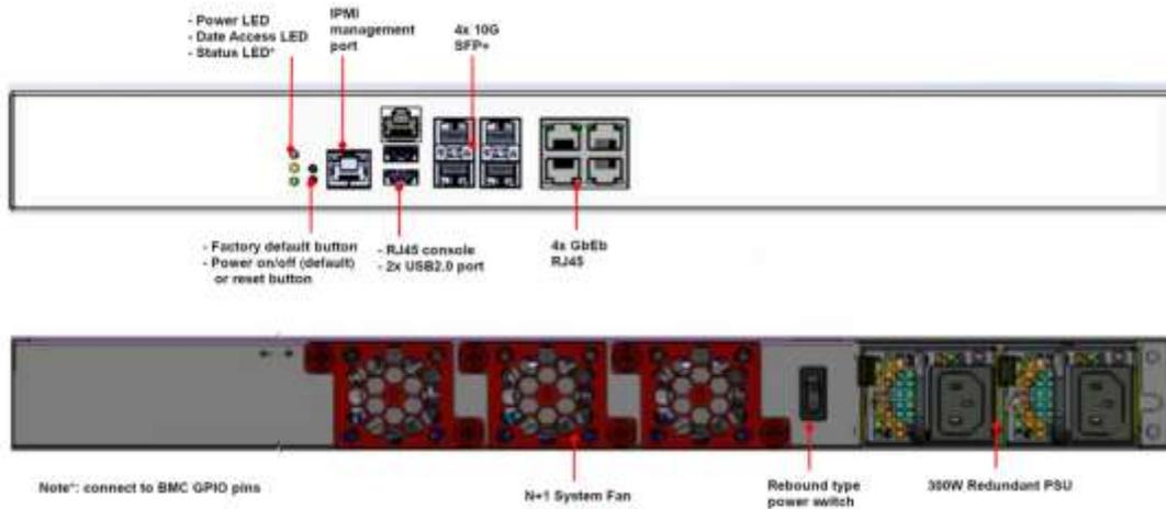
Figure 2: SmartZone 144 Front and Rear View
