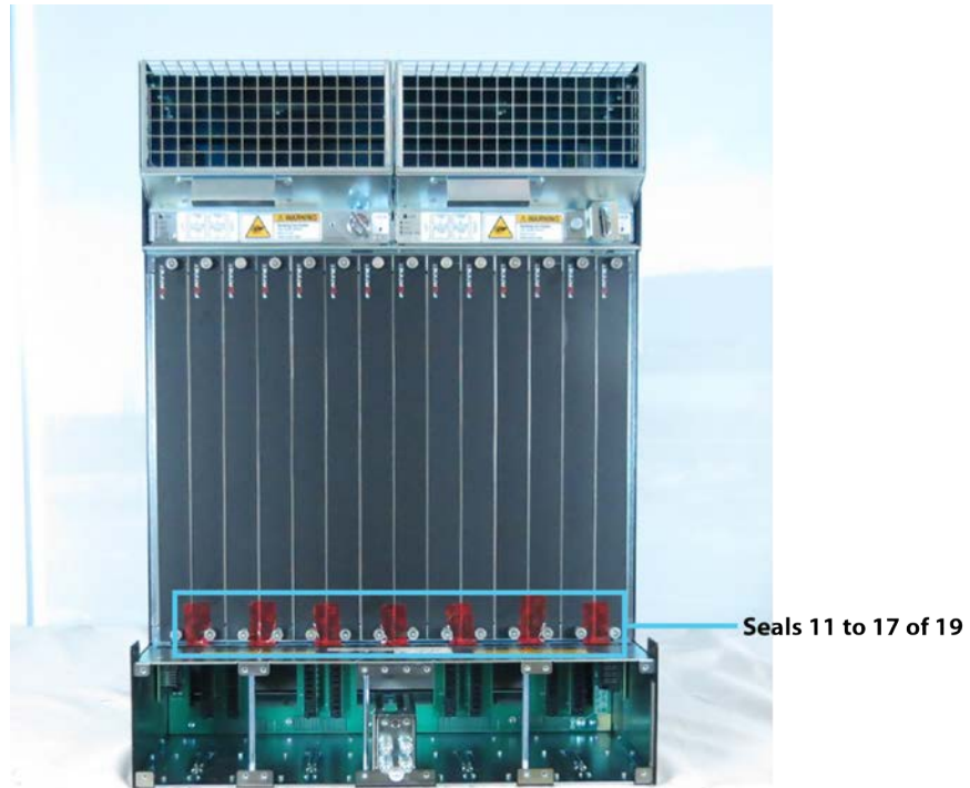
Figure 7 - FortiGate-5001E1 seals, rear view
