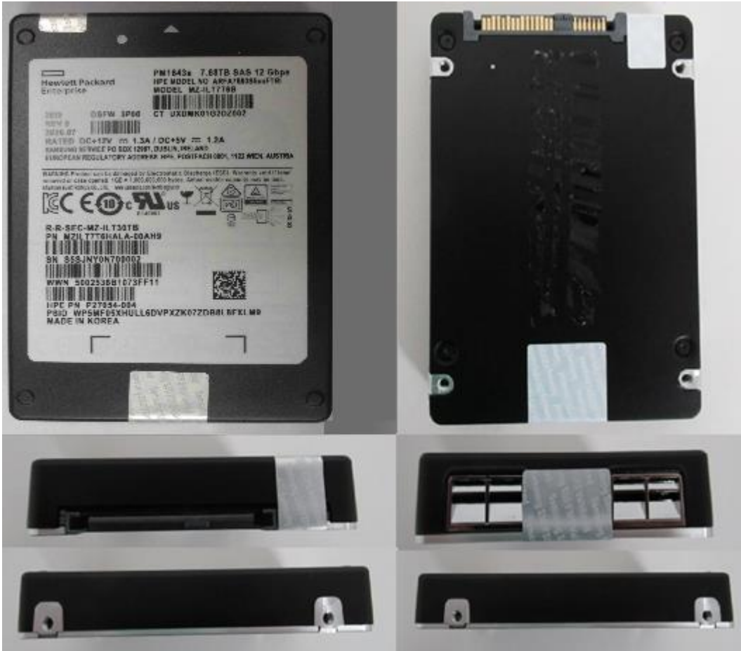
Exhibit 9 – Specification of the Samsung SAS 12G TCG Enterprise SSC SEDs PM1643a Series, MZILT7T6HALA-00AH9, Cryptographic Boundary (From top to bottom – Left to right: top side, bottom side, front side, back side, left side, and right side).
