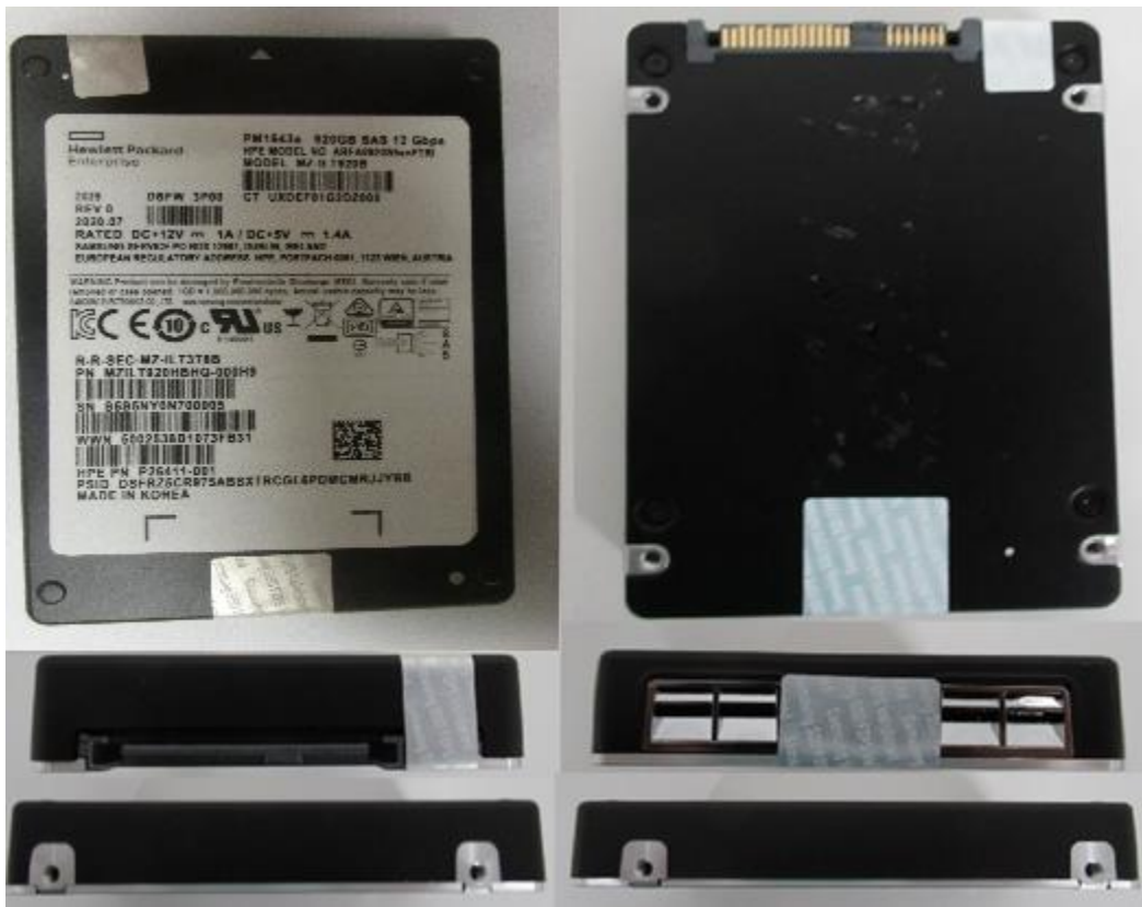
Exhibit 2 – Specification of the Samsung SAS 12G TCG Enterprise SSC SEDs PM1643a Series, MZILT920HBHQ-000H9, Cryptographic Boundary (From top to bottom – Left to right: top side, bottom side, front side, back side, left side, and right side).
