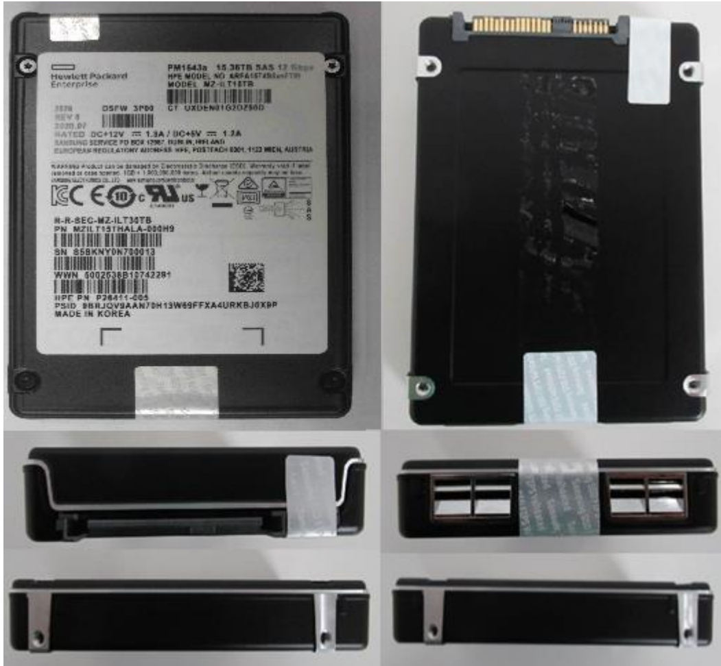
Exhibit 10 – Specification of the Samsung SAS 12G TCG Enterprise SSC SEDs PM1643a Series, MZIL15THALA-000H9, Cryptographic Boundary (From top to bottom – Left to right: top side, bottom side, front side, back side, left side, and right side).
