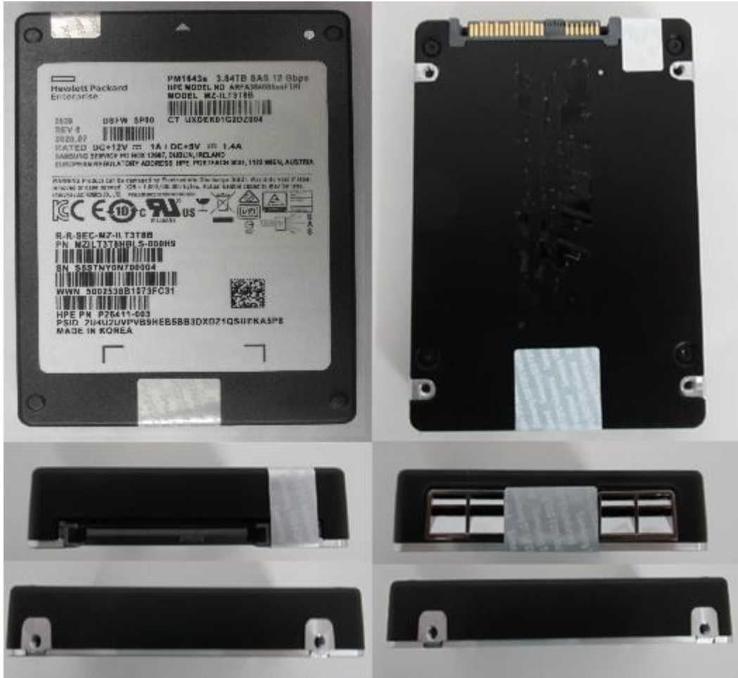
Exhibit 6 – Specification of the Samsung SAS 12G TCG Enterprise SSC SEDs PM1643a Series, MZIL1T3TB8LS-000H9, Cryptographic Boundary (From top to bottom – Left to right: top side, bottom side, front side, back side, left side, and right side).
