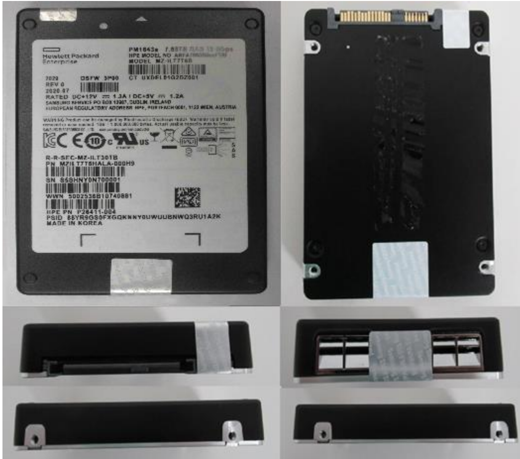
Exhibit 8 – Specification of the Samsung SAS 12G TCG Enterprise SSC SEDs PM1643a Series, MZIL7T6HALA-000H9, Cryptographic Boundary (From top to bottom – Left to right: top side, bottom side, front side, back side, left side, and right side).
