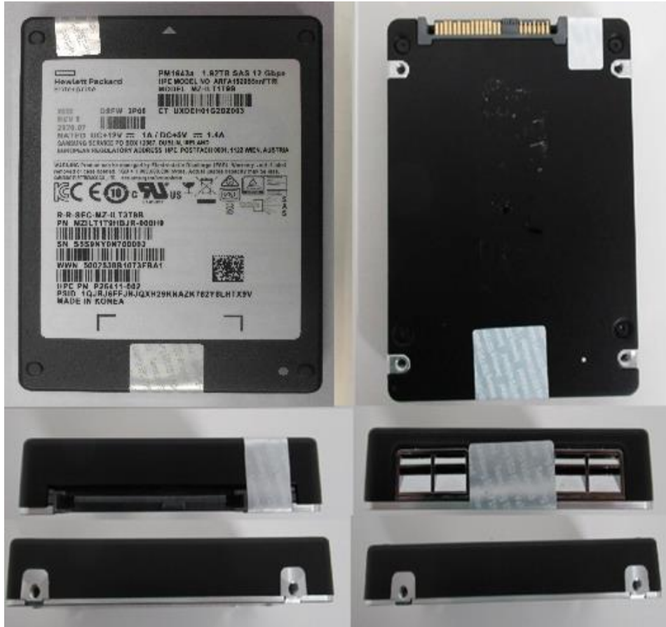
Exhibit 4 – Specification of the Samsung SAS 12G TCG Enterprise SSC SEDs PM1643a Series, MZILT1T9HBJR-000H9, Cryptographic Boundary (From top to bottom – Left to right: top side, bottom side, front side, back side, left side, and right side).
