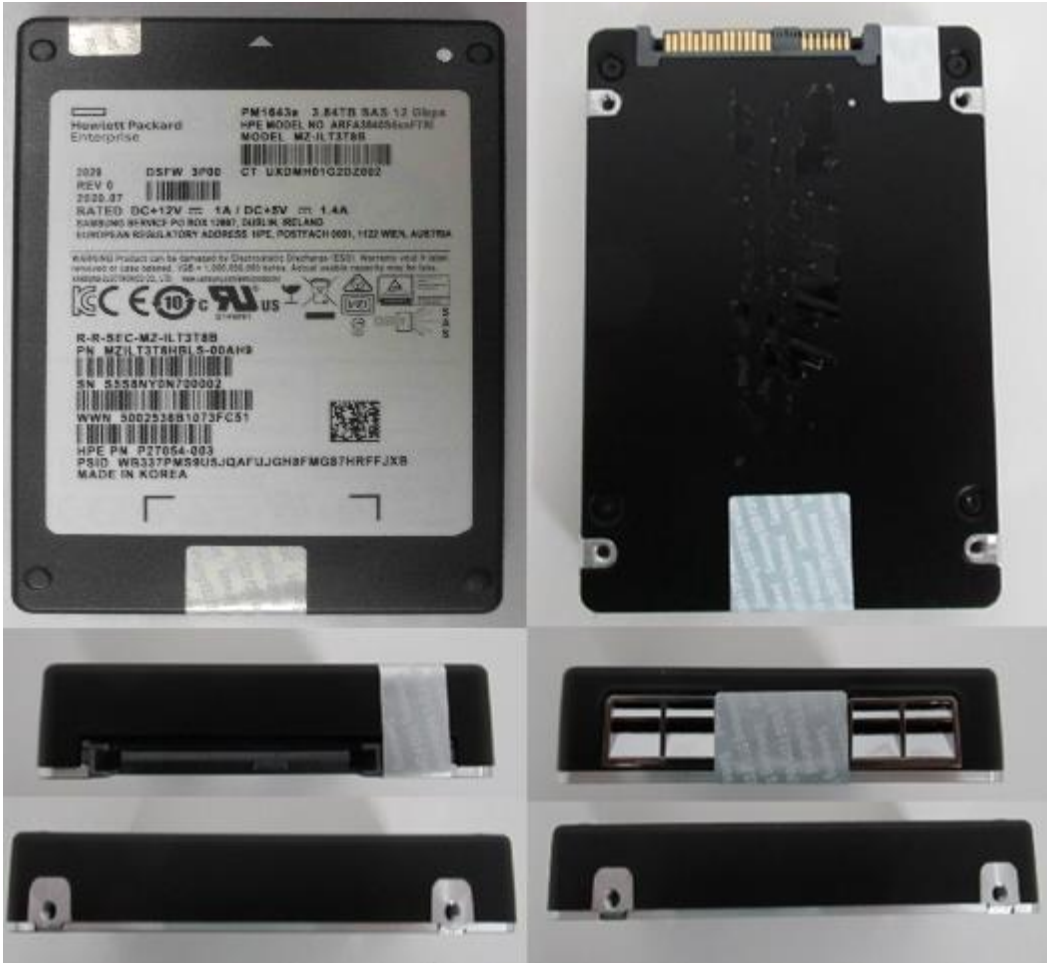
Exhibit 7 – Specification of the Samsung SAS 12G TCG Enterprise SSC SEDs PM1643a Series, MZILT3T8HBL5-00AH9, Cryptographic Boundary (From top to bottom – Left to right: top side, bottom side, front side, back side, left side, and right side).
