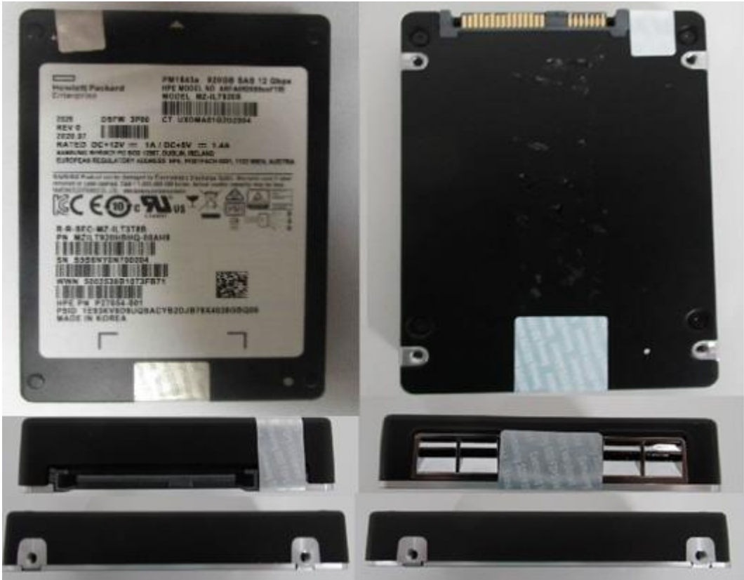
Exhibit 3 – Specification of the Samsung SAS 12G TCG Enterprise SSC SEDs PM1643a Series, MZILT920HBHQ-00AH9, Cryptographic Boundary (From top to bottom – Left to right: top side, bottom side, front side, back side, left side, and right side).
