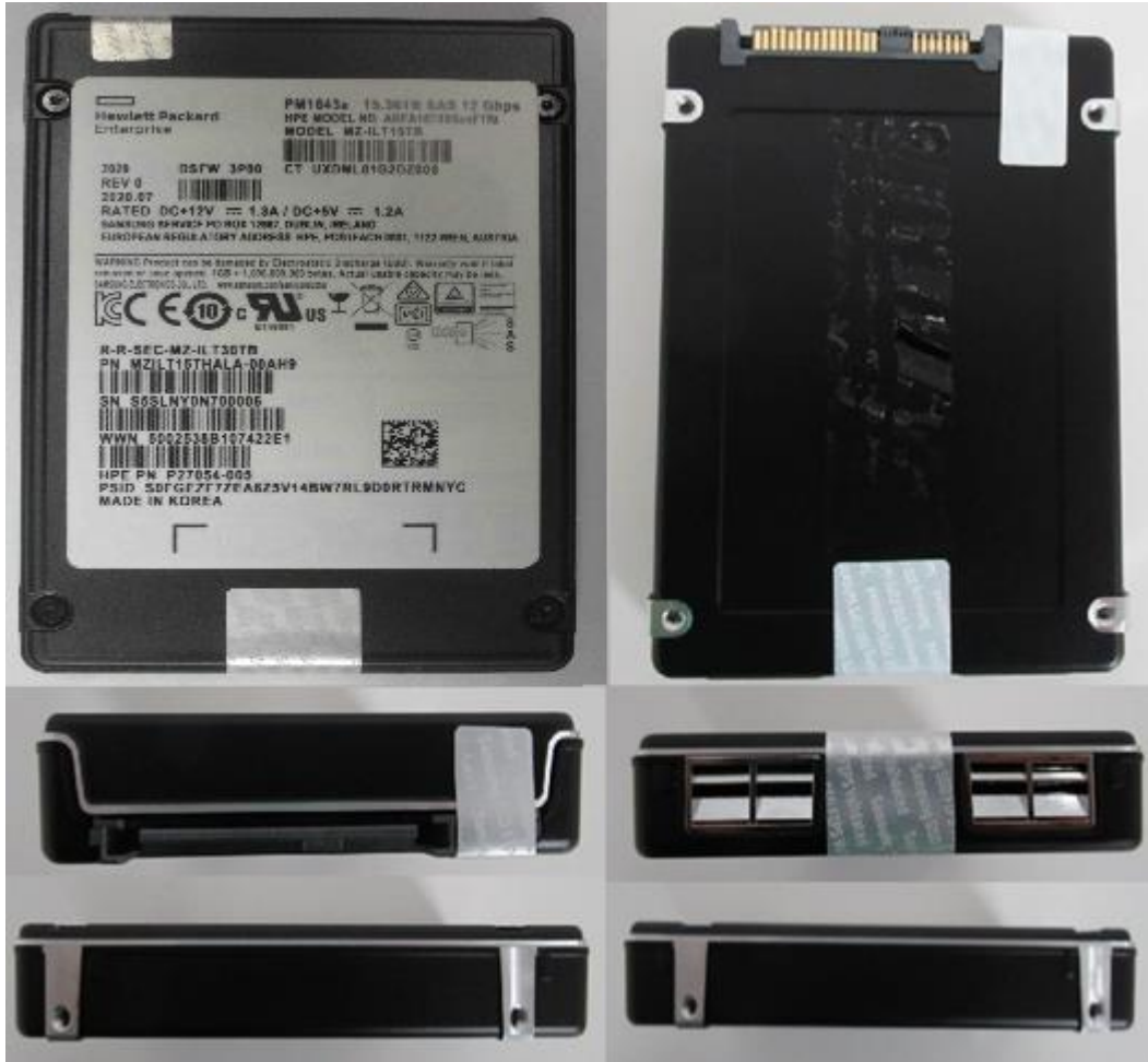
Exhibit 11 – Specification of the Samsung SAS 12G TCG Enterprise SSC SEDs PM1643a Series, MZILT15THALA-00AH9, Cryptographic Boundary (From top to bottom – Left to right: top side, bottom side, front side, back side, left side, and right side).
