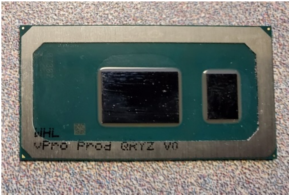
Figure 1a – Intel Cannon Point PCH with Whiskey Lake (WHL) chipset
