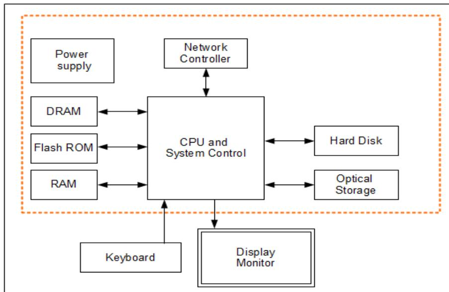
Figure 2: Oracle Linux OpenSSL Hardware Block Diagram
