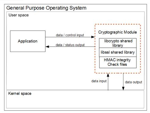
Figure 1: Oracle Linux OpenSSL Logical Cryptographic Boundary
