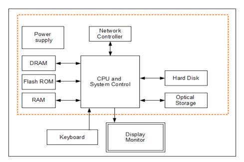
Figure 2: Oracle Linux UEK Hardware Block Diagram
