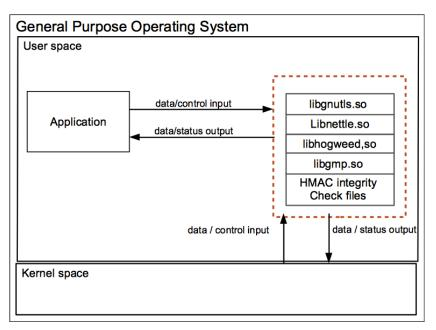
Figure 1: Oracle Linux 8 GnuTLS Logical Cryptographic Boundary
