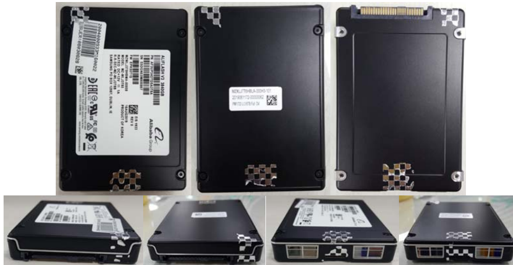
Exhibit 16 – Example of Signs of Tamper
