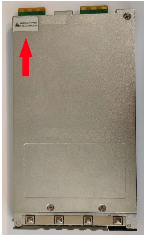
Figure 4 – Tamper-Evident Seal in PALM
