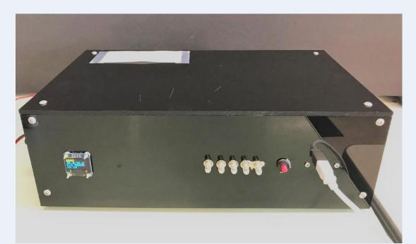
The PSRNG is housed in an insulated box to reduce temperature-induced drift. It has real-time monitoring and communicates with the beacon through a microcontrollerbased USB interface.
