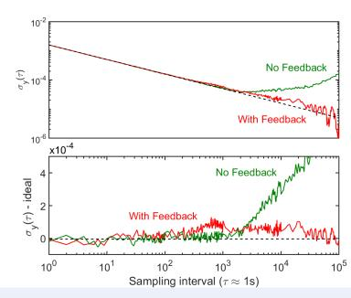
After feedback, output is statistically indistinguishable from white noise (dashed black line) for sample sizes of up to one day.
