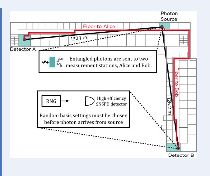
The PSRNG was used in one of the first experimental demonstrations of a loopholefree Bell test [2].
