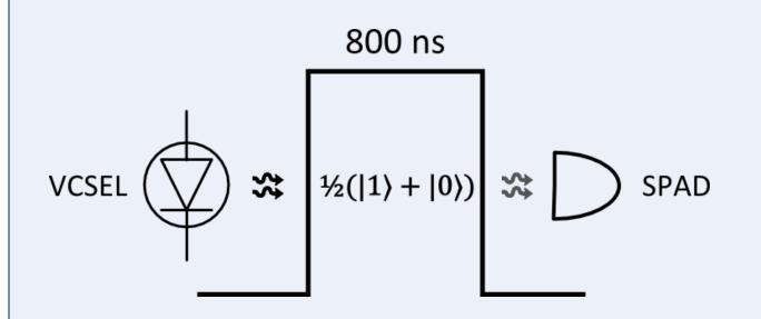
The arrival time of single photon from a coherent source is a random process. Bit values are determined by whether a photon is detected during an 800 ps window.
