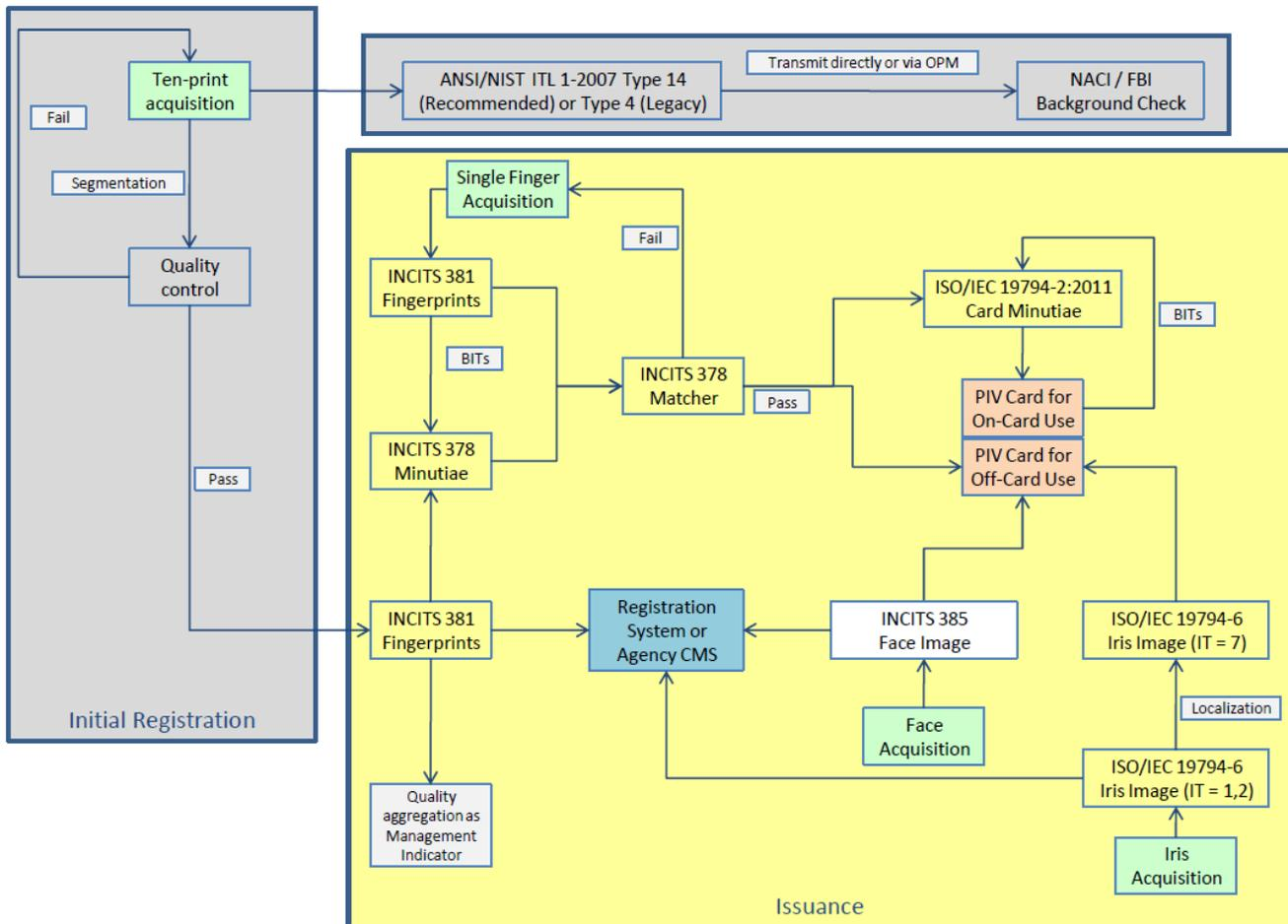
313 **Figure 1 – PIV biometric data flow**
