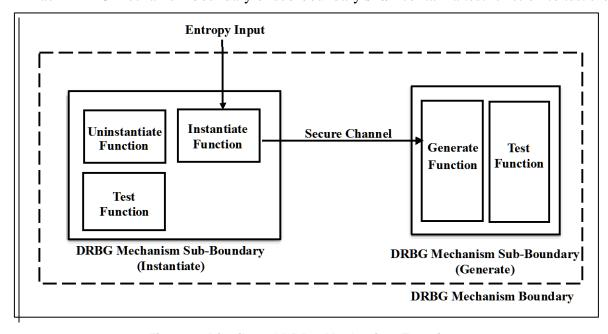
Figure 4: Distributed DRBG Mechanism Functions
