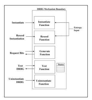
Figure 3: DRBG Mechanism Functions within a Single Device
