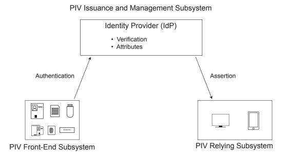
Figure 3-4. PIV System Federation Connections
