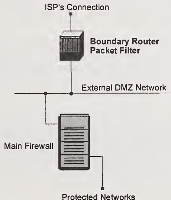
Figure 2.4: Packet Filter used as Boundary Router
