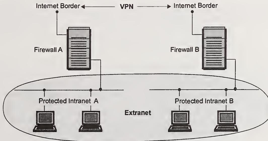
Figure 3.4: VPN/Extranet Joining Two Intranets
