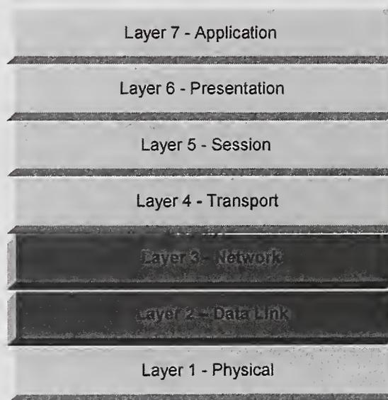
**Figure 2.3: OSI Layers Addressed by Packet Filters**
