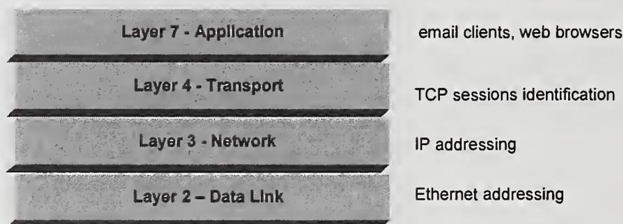
**Figure 2.2: OSI Layers Operated on Modern Firewalls**
