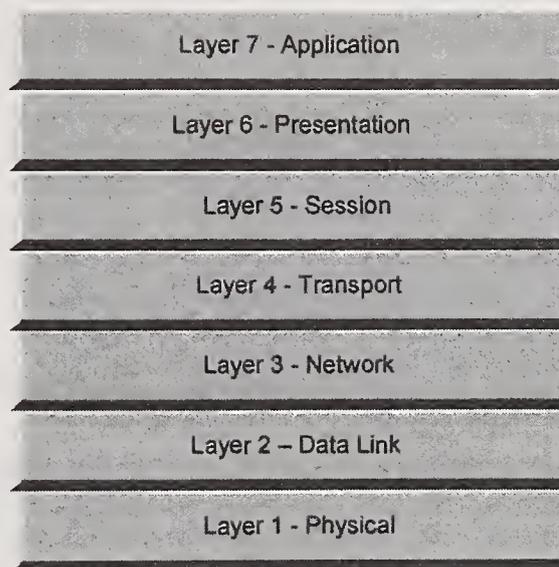
Figure 2.1: OSI Communications Stack
