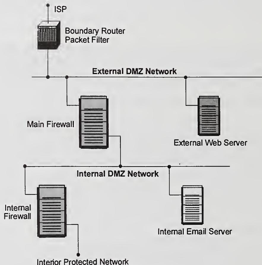
Figure 3.1: A DMZ Firewall Environment
