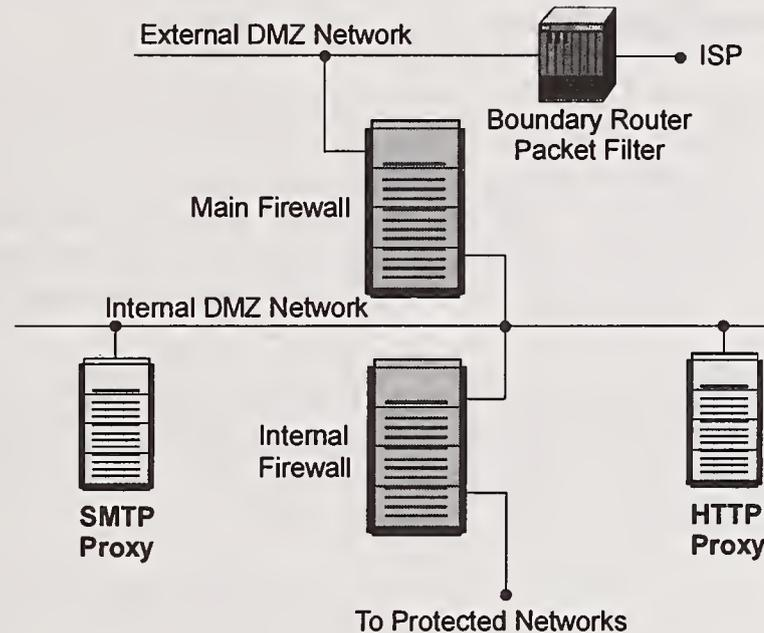
Figure 2.8: Application Proxy Configuration
