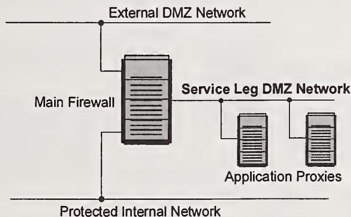
Figure 3.2: Service Leg DMZ Configuration
