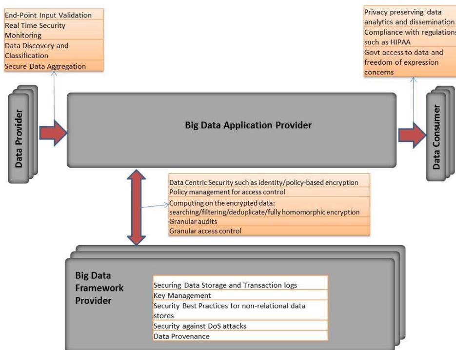
Figure 6: Notional Security and Privacy Fabric Overlay to the NBDRA
